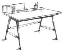
Desk Folding top in birch plywood and oak veneer. Black steel structure. W. 110 D. 60 H. 75
